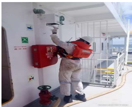
4EO confirming all vents closed.
