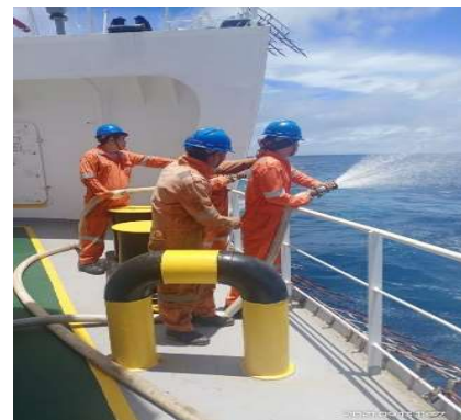
Boundary cooling in progress.
